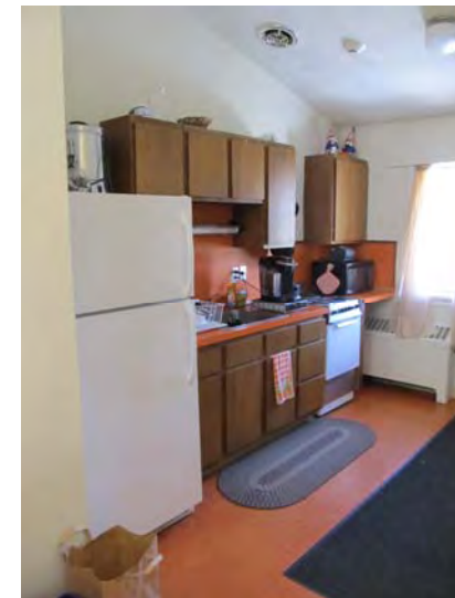
Community kitchen – Note lack of knee clearance space under sink and a thirty-inch wide work surface
